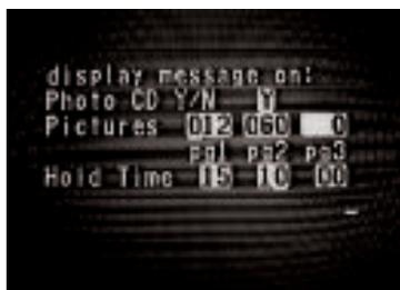
The Kid CG can control a Photo CD player and put messages over the images it produces. You can link a message to a specific Photo CD image, creating a Text/Image Combination. This window tells the VM-1FS what image to retrieve from the CD player before playing the message. Three images can be linked to the three individual pages with a message.
