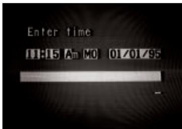
**SETTING THE CLOCK:** This screen allows you to set the time, day of week and date. The clock affects all the timing and scheduling functions in the Kid. Again, use the Arrow Keys to position the cursor, make your entry, then press the Enter Key.
