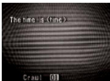
Please note the Time and Date commands. The commands (time) and (date) in brackets can be inserted into any text string. The commands can be used in the header, message or crawl areas of the display. When the text plays in which these commands are used, the Kid CG will insert the current time and or date as designated.
