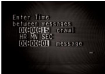
**TIME BETWEEN MESSAGES:** This screen allows you to set the time interval you wish between crawl and message presentations. This interval can be set from 2 seconds to 99 hrs., 59 mins., 59 seconds (see window in the left margin). This instruction applies to all 90 messages and 20 crawl lines. Use the Arrow Keys to position the cursor, make your entry, then press the Enter Key.
